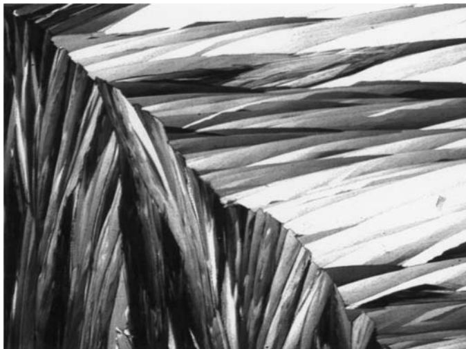
FIG. 1—Fusion preparation of TNT viewed with crossed polars.
